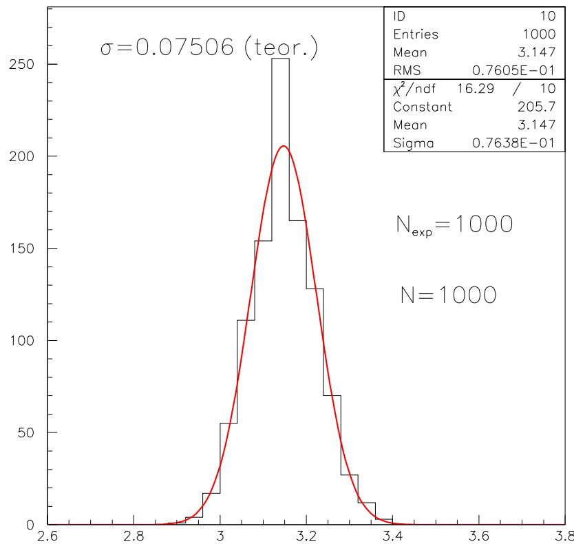
$$\bullet \sigma_I = \frac{\pi}{2} \frac{\sigma_m}{N} = \underbrace{\frac{\pi}{2} \frac{m}{N}}_{\approx 1} \frac{\sigma_m}{m} = \frac{\sigma_\pi}{\pi}$$
