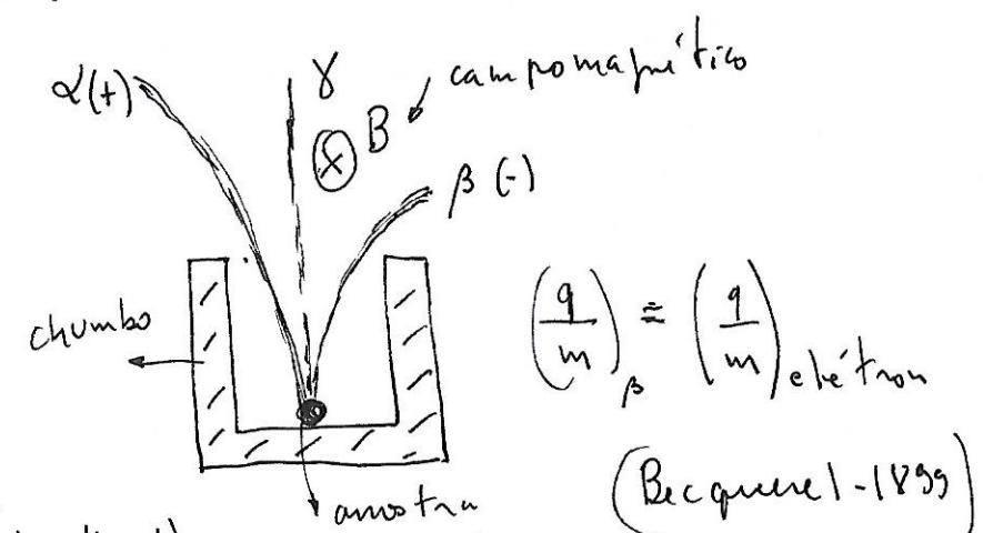
$$\left(\frac{q}{m}\right)_{\alpha} = \frac{1}{2} \left(\frac{q}{m}\right)_{H^+} = \frac{1}{2} \left(\frac{e}{m}\right)_{proton}$$
