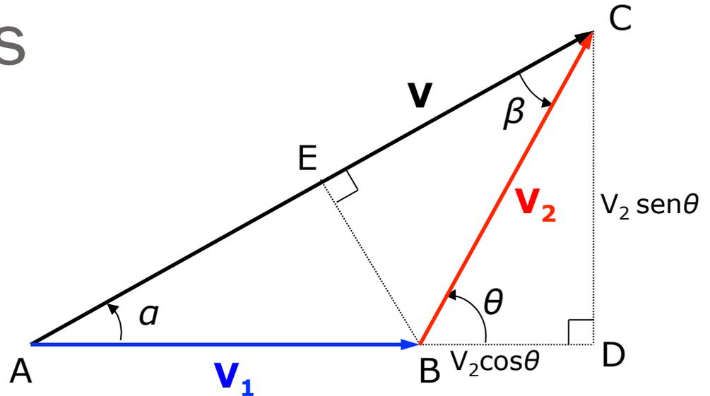
$$CD = AC \operatorname{sen} \alpha = BC \operatorname{sen} \theta \quad \Leftrightarrow \quad V \operatorname{sen} \alpha = V_2 \operatorname{sen} \theta \quad \text{ou} \quad \frac{V}{\operatorname{sen} \theta} = \frac{V_2}{\operatorname{sen} \alpha}$$
