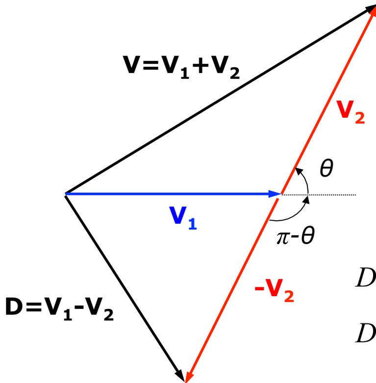
$$D = \sqrt{V_1^2 + V_2^2 + 2V_1V_2 \cos(\pi - \theta)}$$
